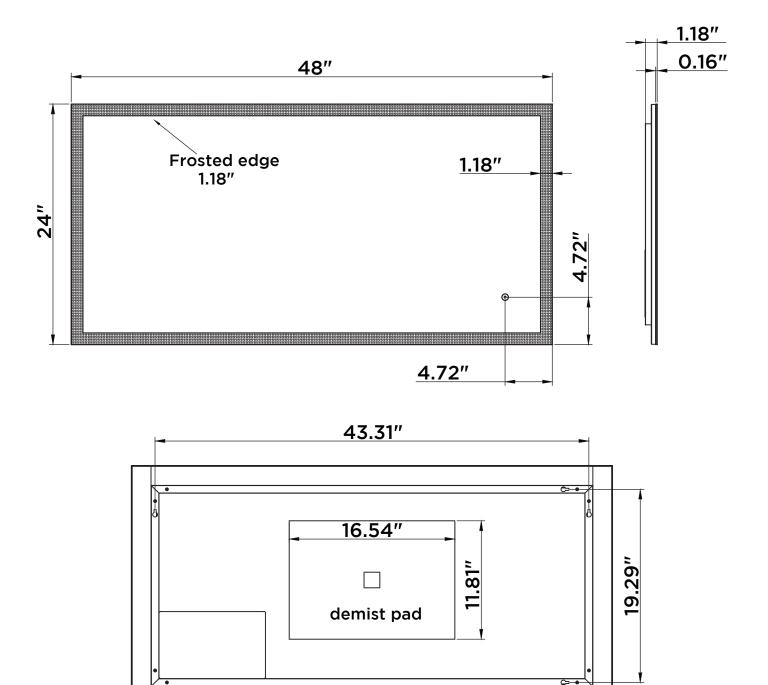
**ATTENTION!** Dimensions may vary by up to 3/8". It is highly recommended to pull all dimensions of actual model for installation and measuring purposes.
